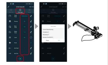
Time-lapse shooting  $\rightarrow$  Set key points  $\rightarrow$  Set starting point and ending point  $\rightarrow$  Set other parameters  $\rightarrow$  Whether to go back and forth  $\rightarrow$  Choose yes and click start  $\rightarrow$  Slider moves from current position to "starting point" position  $\rightarrow$  Start to execute action, every time pause and take a picture, until all the setting number of pictures is taken.
