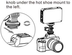
6 Rotate counterclockwise to loosen the angle fixing knob of the hot shoe mount, adjust to the appropriate angle, and then tighten the angle fixing knob clockwise to fix the angle of the light.
