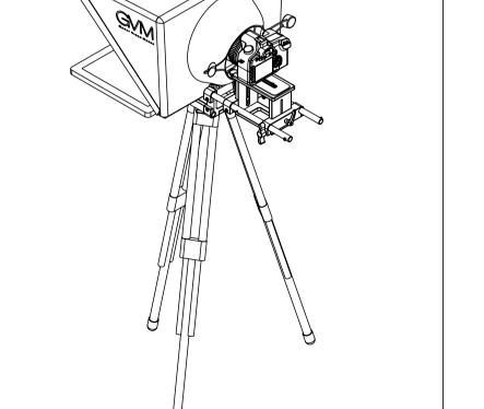
7 As shown in the figure below, install the 'camera' to the 'camera bracket'.
