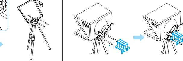
6 As shown in the figure below, first loosen the screws at the back of the 'base',
