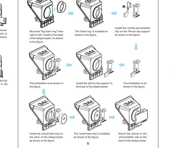
Horizontal recording with mobile phone, the installation method is as shown
