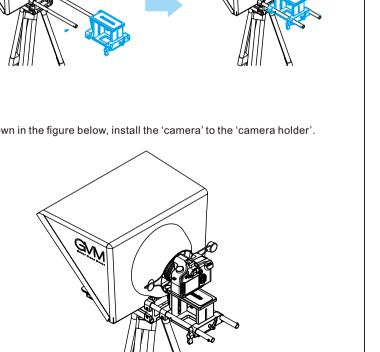
7 As shown in the figure below, first loosen the screws at the back of the 'base',
