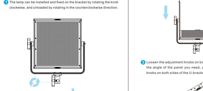
3 Loosen the adjustment knobs on both sides of the U-bracket, adjust the angle of the panel you need, and then tighten the adjustment
