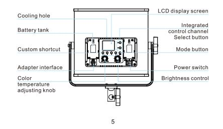
1 The lamp can be installed and fixed on the bracket by rotating the knob clockwise, and unloaded by rotating in the counterclockwise direction.
