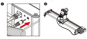
5) Install the battery on the slider and check the signal cable or shutter cable connecting correctly or not. (As shown below)
