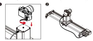
${\bf 4}$  ) Use the shutter cable to connect the motorized camera head and camera. (As shown below)
