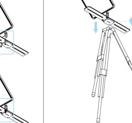
As shown below, install the teleprompter base to the tripod.
