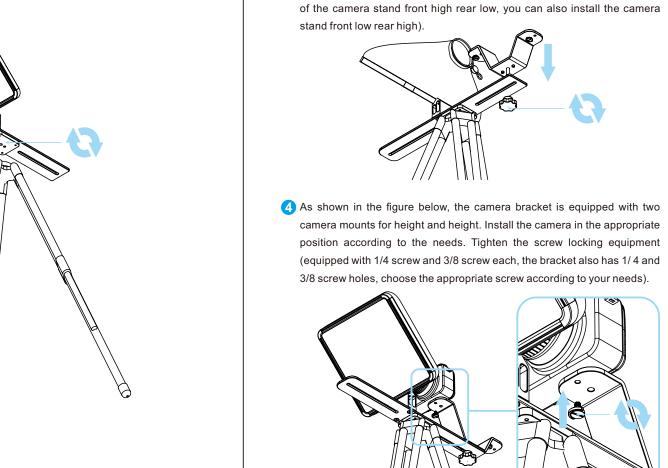
3 As shown in the figure below, attach the camera bracket to the base and
