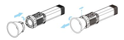
Insert the bowen's adapter into the socket of the light accordingly, and then turn it slightly clockwise to lock the Bowen's adapter to the light. Push the slider back and rotate the Bowen's adapter counterclockwise to remove it from the light.
