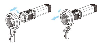
3 Turn the knob clockwise to fix the lamp on the handle, turn it counterclockwise to remove it.
