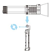
4 Loosen the knob to adjust the Angle of the lamp, and tighten the knob after the Angle is adjusted.
