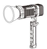
**5** Loosen the knob to adjust the Angle of the lamp, and tighten the knob after the Angle is adjusted.
