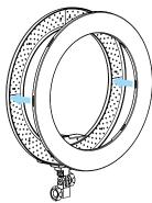
3 Loosen the knob on the left of the bracket, adjust the angle you need, and then tighten the adjustment knob on the left of the bracket.
