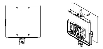
Install the external Diffuser: install the diffuser support frame to the lamp, align the diffuser with the screw hole, and lock the diffuser with the screw.
